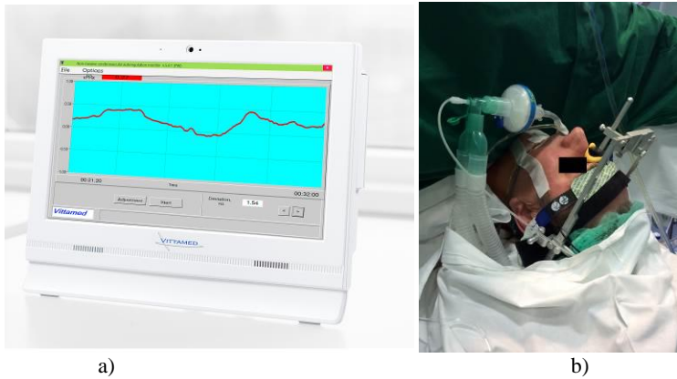
Fig. 1. The Vittamed 505 non-invasive CA monitor (a), the mechanical frame with ultrasonic transducers mounted on the patient’s head during cardiac surgery with CPB (b).
