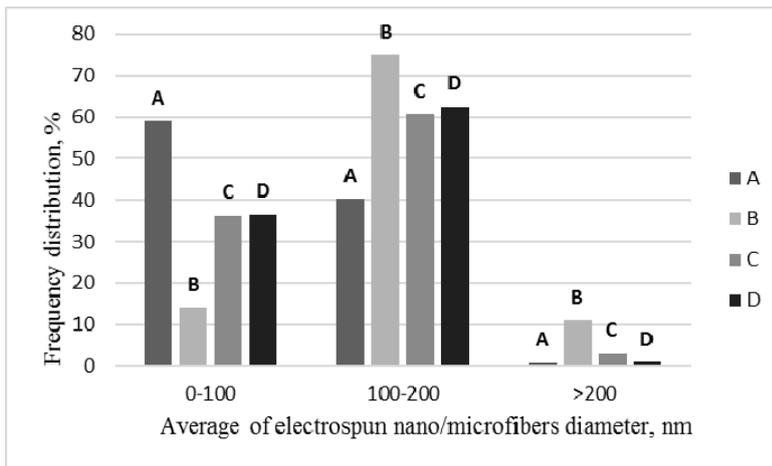
**Fig. 2.** The distribution of electrospun PVA nano-microfibers diameter with HAp powders (A - HAp powders, B - BHA powders, C - HAp powders sintered at 1000 °C, D – BHA powders sintered at 1000 °C)
