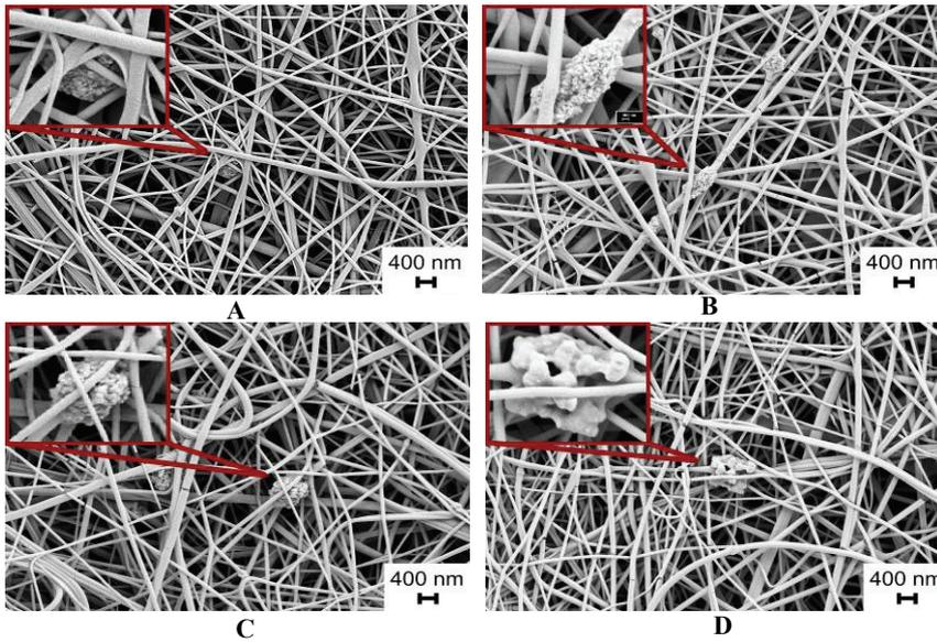
**Fig. 1.** SEM images of electrospun mats from PVA nano-microfibers with HA (the amount of HAp powder in electrospun solution is 5 wt%): A - HAp powders, B - BHA powders, C - HAp powders sintered at 1000°C, D – BHA powders sintered at 1000°C.
