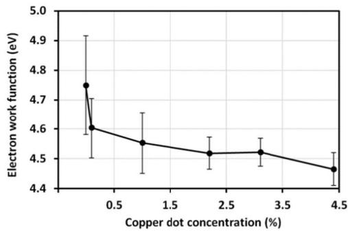
Fig. 3. The value of  $\phi$  of Titanium oxide nanofilm coated the Ti substrate in dependence on the embedded Cu nanodots density [9]
