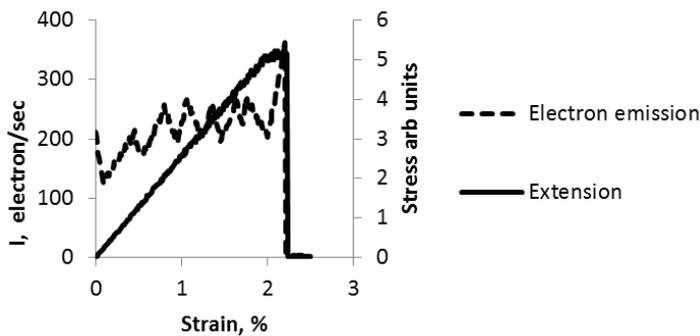
Fig. 1. Strain and electron emission diagrams of the composite material (epoxy binder mixed with carbon nano tubes) [5]
