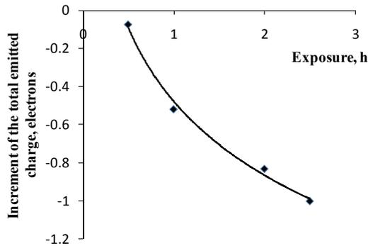
Fig. 4. Emitted charge increment versa exposure in benzene gas [12]
