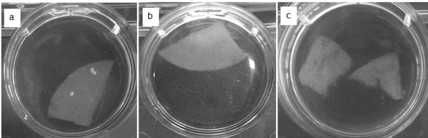
Fig. 4. Structural stability and degradation *in vitro* of coated HA scaffolds after 1 day (a), 2 weeks (b) and 2 months (c) of immersion
