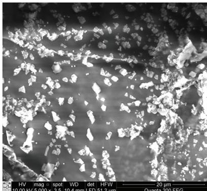
**Fig. 2.** SEM micrograph of the surface of HA scaffold coated with SiO<sub>2</sub>
