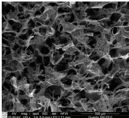
**Fig. 1.** SEM image of highly porous HA scaffold
